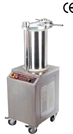
SF-260 Dimension(LxWxH): 640x485x1240mm Voltage: 220V/50Hz Power: 0.75Kw Bowl dia: Φ 260mm Productivity: 400kg/h Bowl Volume: 17L N.W: 90kgs
